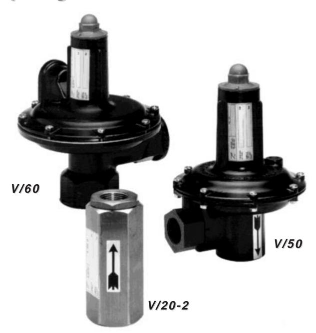
The automatic spring-loaded relief valves are designed to keep line pressure below preset values. They are mounted downstream of regulators and perform the specific function of releasing small amounts of gas in the event of the regulator not closing perfectly.
