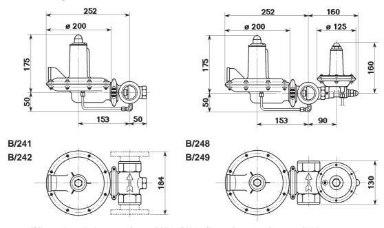
11/2" gas threaded connections - DN 40 PN 16 flanged connections available on request.
