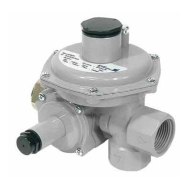
The **DKR** series regulators are a line of direct action type pressure regulators, <u>double stage</u>, normally for domestic use directly assembled to the meter or in decompression installations for civil and industrial uses in canalized networks for natural and manufactured gas, Lpg or other non corrosive, preliminarily treated stable gases.
